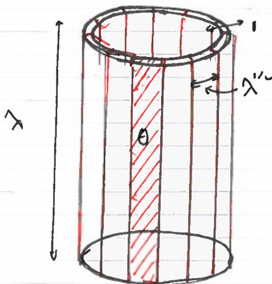
The cylinder and corresponding plate decomposition.
