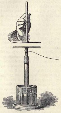
the zinc plate where the copper was, and the copper where the zinc was. This time we are to observe the electrification of the copper plate when it has come in contact with the zinc. I make the contact, and with308
