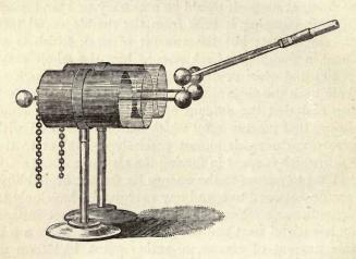
to judge roughly the amount of work which corresponds to its full charge by the sound and light of the spark. After that I shall charge it again as nearly as possible to the same amount, and then share the charge of electricity between the two jars, by putting first their outer coatings together, and then their inner coatings; so that the charge shall be divided equally (because of their equality) between the two. You now obtain (showing) from the sound and light of that discharge-
