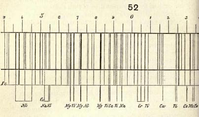
one-half of the slit of the spectroscope, and light from incandescent materials (in the electric arc or in an induction spark, or even a Bunsen lamp) through the remaining half, and examine them through the same train of prisms, you get two spectra as here represented, the one of sunlight and the other of the terrestrial substance, spread out side by side. Any two rays which, in passing through a very long series of prisms, undergo
