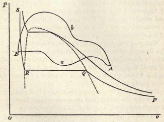
given temperature water begins to form. Then, however much more we may compress up to a certain limit, the pressure does not alter, so that our curve then runs along parallel to the horizontal line, and it does so until all the steam is converted into water; and then by further application of pressure we compress the water; —but exceedingly little—so that in reality our curve is almost a straight line running vertically upwards.
