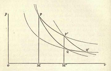
stant is proportional to the pressure in the cylinder at that instant. To fix the ideas, suppose the cylinder to be horizontal, and the just-mentioned transverse motion vertical. Then any re-entrant line whatever may be supposed to be traced, once over in each cycle of the engine, by the pencil P. For reasons to be afterwards explained, I take the curvilinear quadrilateral PP'Q'Q. Let Ov be the axis of the cylinder, Op perpendicular to it; and let PM be perpendicular to Ov. Then, by our
