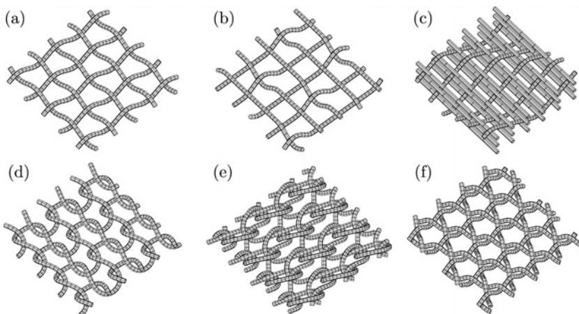
**Figure 1** Examples of textile structures: plain weave (a); sateen (b); multi-layered woven fabric (c); single jersey (d); warp knit (e); triaxial woven fabric (f).
