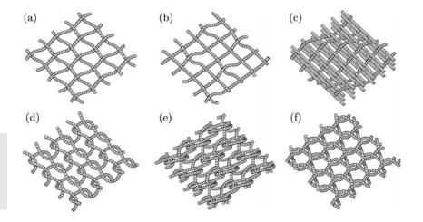
Figure 1 Examples of textile structures: plain weave (a): sateen (b): multi-layered woven fabric (c): single jersey (d): warp knit (e): triaxial woven fabric (f).
